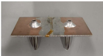
①Copper foil 0.035mm Copper plate 1.6mm (Banana Plug + Banana Jack)
